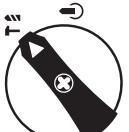
Position for **hammer drilling**. When the drilling tool does not immediately rotate upon switching on, allow the machine to run slowly until the drilling tool rotates.
