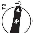
**Vario-Lock** position for adjustment of the chiselling position.
