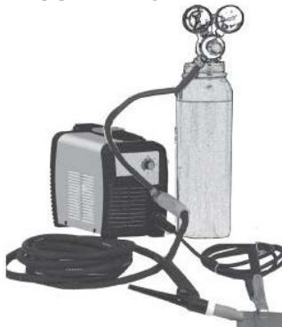
After opening the gas supply using the tap on the torch grip, regulate its flow via the tap on the gas cylinder (app. 6 litres per min.).
